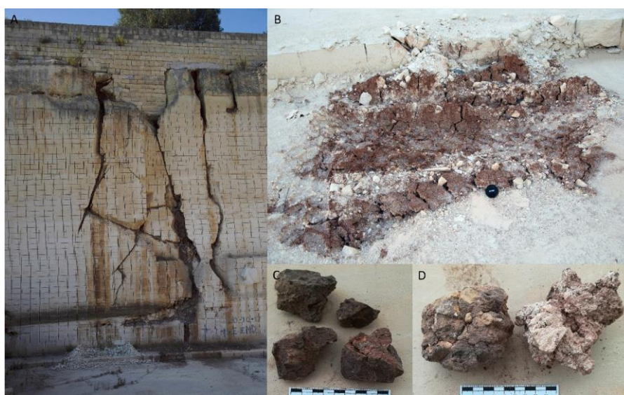
Figure 26. (A) Wall of a Pietra Leccese quarry in Cursi. The fractures are hosting the pocket rich in phosphates and Fe oxides. (B) Closer view of a P-rich pocket. The samples C1 (C) and C2 (D) belong to one of those pockets
